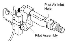
Figure 30 - Pilot Inlet Air Hole
